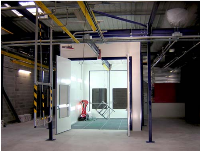
Cabine à ventilation verticale, manutention par transbordeur Booth with vertical ventilation, polymerization oven, handling with transfer rail
