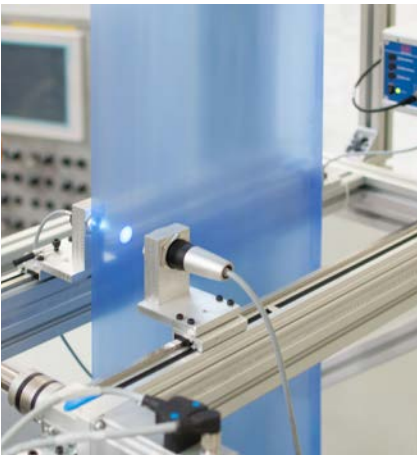
Inline measurement of the colour gradient of glass, Plexiglas, PET and PVC foils, paper.
